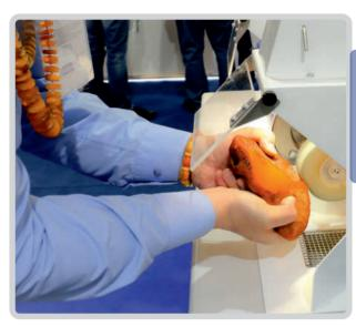
Polishing benches can be used for manual grinding or polishing of small items, semi-finished goods or other jewelry workpieces. Buffing machines are essential for every jewelry workshop and are very useful for workpieces, which cannot be mass finished. Our polishing benches are equipped with integrated exhausting system for processing dust. There is no need to connect it to external exhausting or ventilation system.
