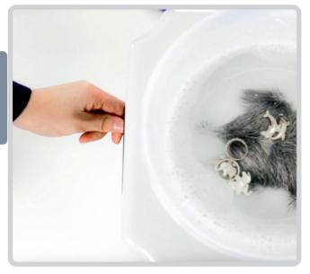
Access to grooves and small corners on the workpiece is often very limited. Preliminary cleaning and polishing of hard accessible corners can be done with magnetic polisher. Magnetic finishers are suitable **for pre-processing of silver and gold workpieces**. Oxidation from previous processes can be easily removed.
