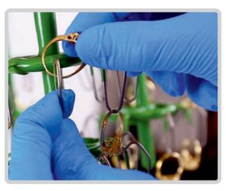
Electropolishing is an electrochemical process that removes the outer layer of material on a metal part **without rounding the edges**. It offers a **unique advantage** of treating the areas on the workpiece, which are not approachable by the common mechanical process. Moreover the finishing effect can be achieved in a very short time -from 5 to 35 min.
